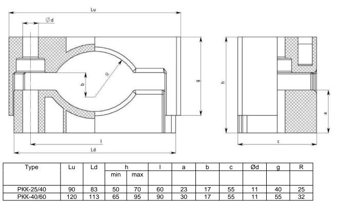
Figure 1. External appearance and overall dimensions (mm)
